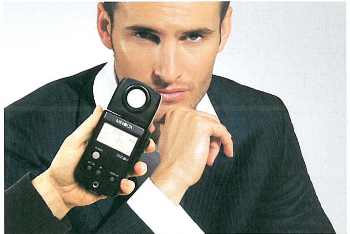
△ Close-up Place the meter as close to the subject as possible to take the most accurate readings.
