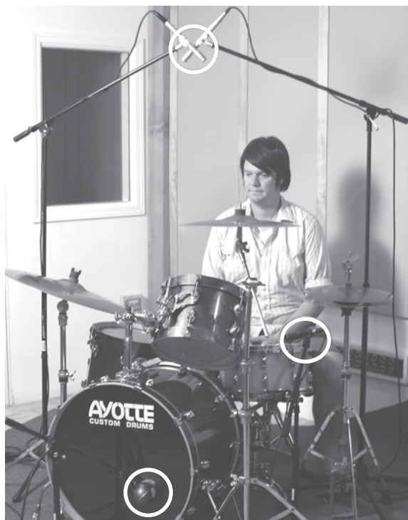
Figure 8.16 Four-mic technique with ORTF overheads.
