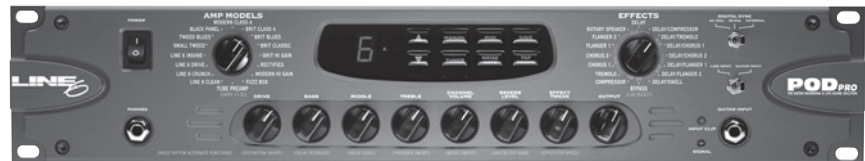
Figure 3.15 An amplifier emulator: Line 6 Guitar POD Pro. Courtesy of Line 6.
