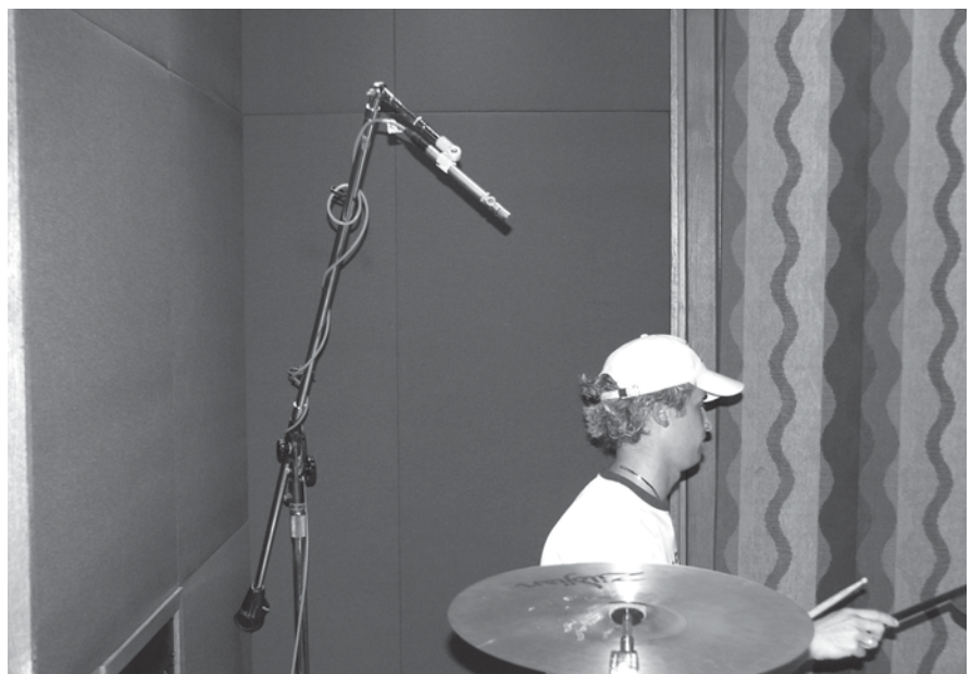
Figure 8.15 Small-diaphragm condenser behind the drummer, pointed at snare and hat.
