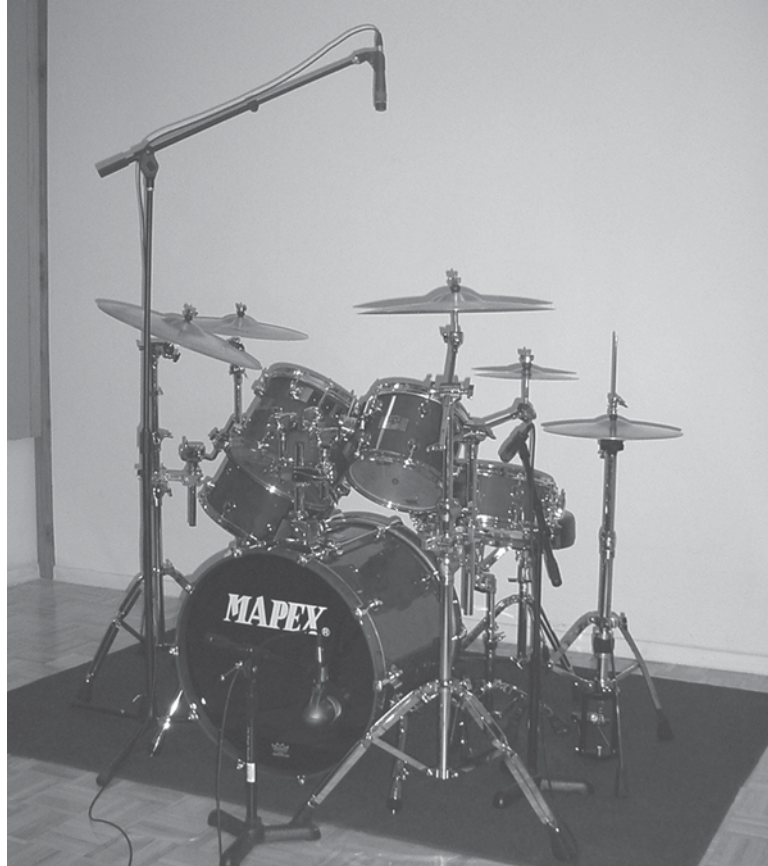
Figure 8.12 Three-mic configuration using overhead, snare, and kick drum mics.
