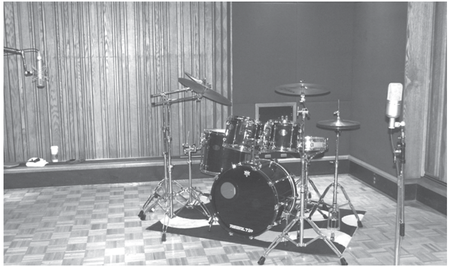
Figure 8.10 U 47 and M 149 in two-mic configuration in front of the drums.
