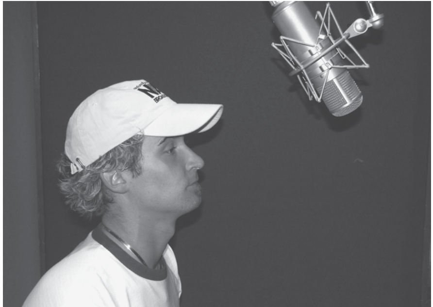
Figure 8.66 Alternate vocal mic placement using a large-diaphragm condenser mic.
