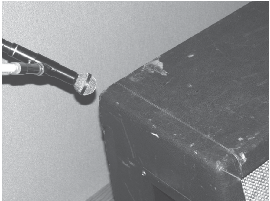
Figure 8.51 Beyer M160 on Marshall cabinet corner.
