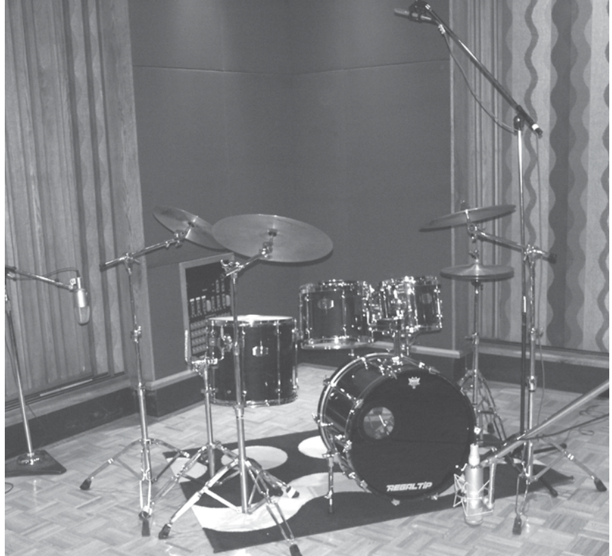
Figure 8.13 Three-mic setup: M 149 on left, U 47 in front, and Royer R-121 overhead.
