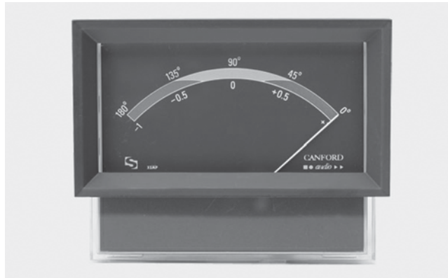
Figure 6.5 A phase meter with an in-phase signal.
