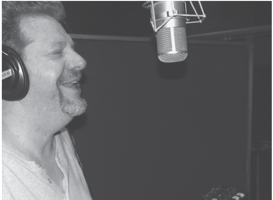
Figure 8.65 Vocal mic placement using a large-diaphragm condenser mic.
