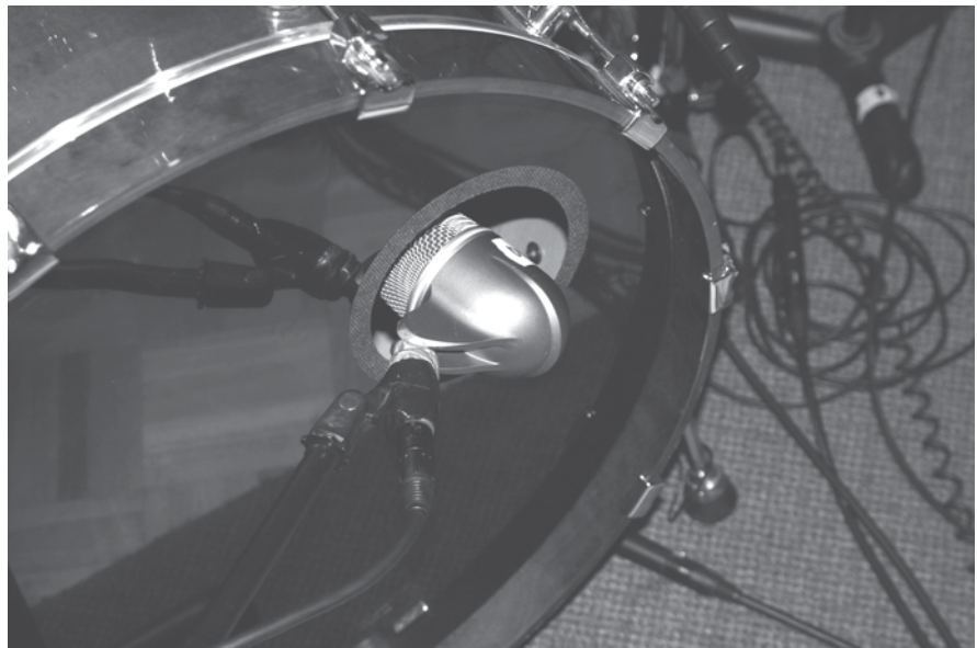
Figure 8.17 AKG D 112 just inside the hole.
