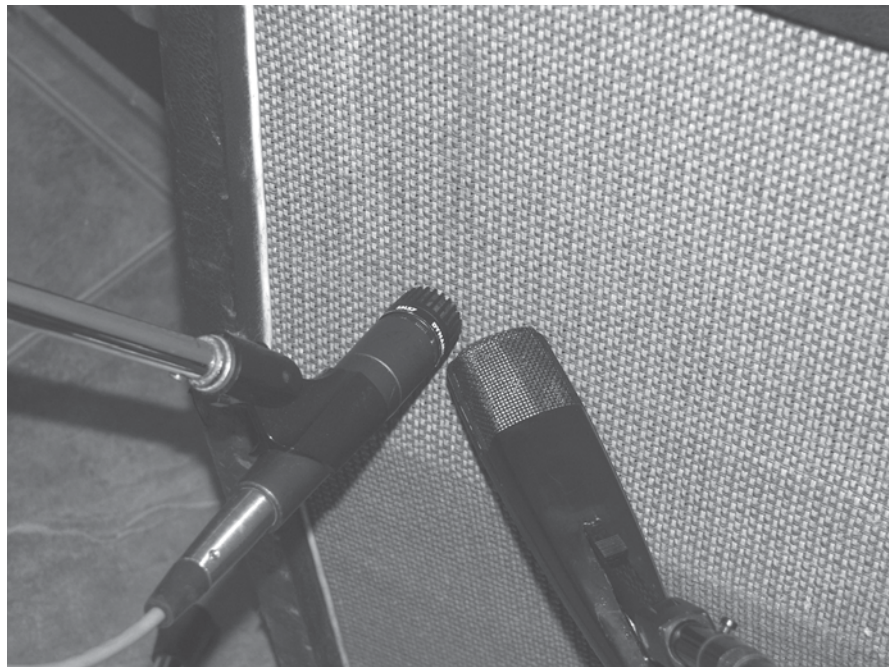
Figure 8.48 SM57 And Sennheiser MD421 on guitar cabinet.
